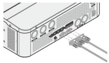
See the diagram below for parallel connection
